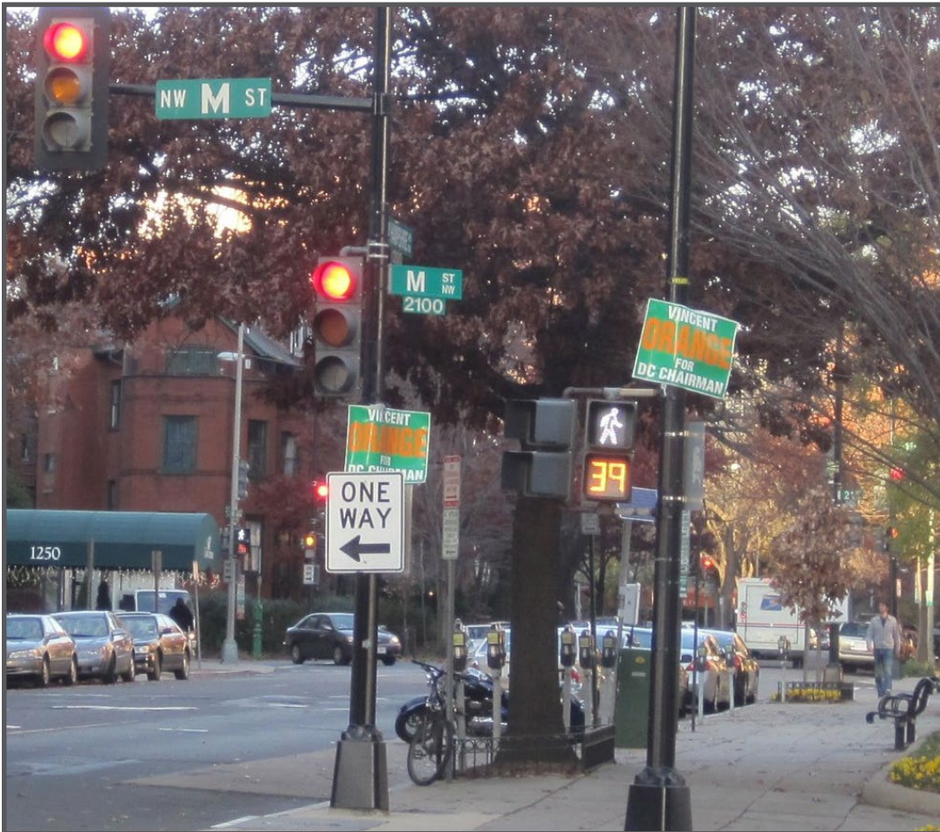
Pedestrians are provided with a leading interval on M Street, Washington D.C.
