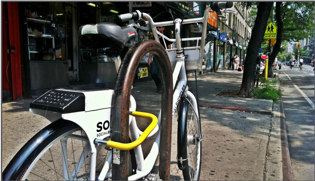
Bike share systems with smart lock technology require no physical docking stations.
